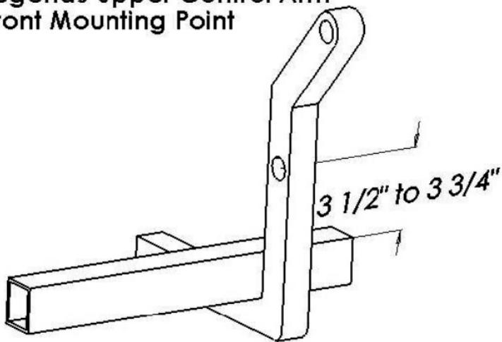
**3 1/2" to 3 3/4" (from the top of the frame to the center of the pick-up point holes)**
