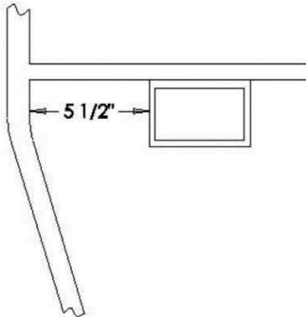
**Note:** The measurement for the battery box offset will be taken at the point closest to the crossmember, from the inside of the framerail to the outside of the battery box.
