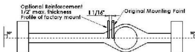
(This reinforcement will secure the opposite side of the rod end of the upper link)
